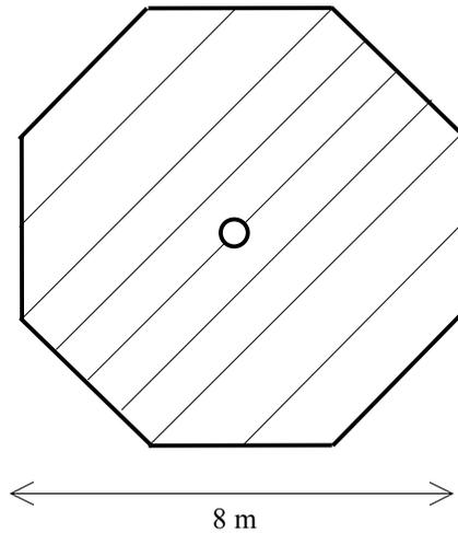
**Fig. 4.** Layout of scintillator modules on a plane of the Far Detector; there are 4 modules containing 20 scintillator strips and 4 (angled) with 28 strips. The 55 cm diameter central hole accommodates the magnet coil.
