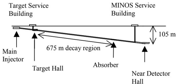
**Fig. 2.** The beamline at Fermilab
