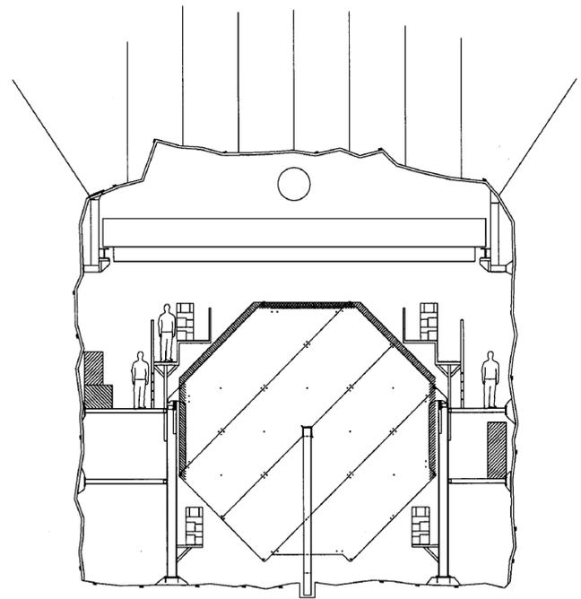
**Fig. 3.** Front view of a hanging steel plane, showing the support structure and the vertical magnet coil.
