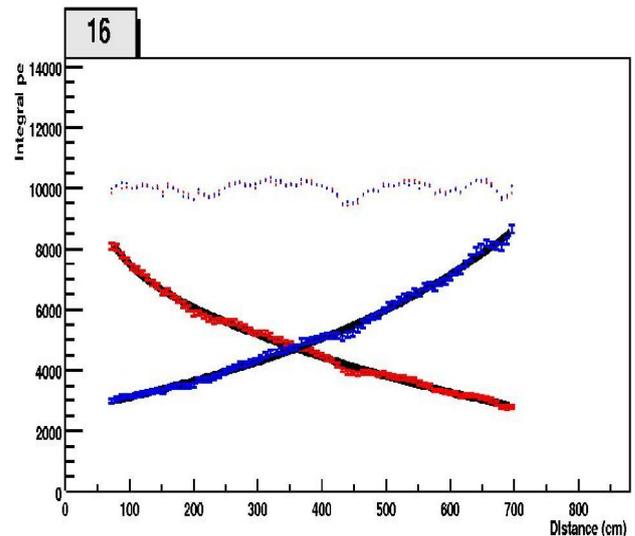
**Fig. 5.** Response map of strip 16 in a typical 8-m long scintillator module.
