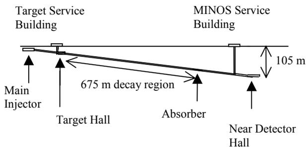
**Fig. 2.** The beamline at Fermilab
