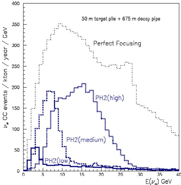
**Fig. 6.** CC event rates for the 3 possible beams; “perfect focusing” refers to the idealized situation where all produced mesons are focused down the beamline without loss.
