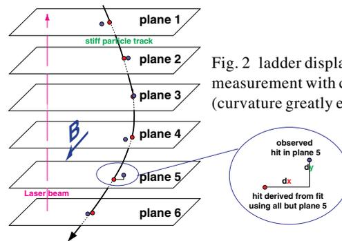
Fig. 2 ladder displacement measurement with cosmic tracks (curvature greatly exaggerated).
