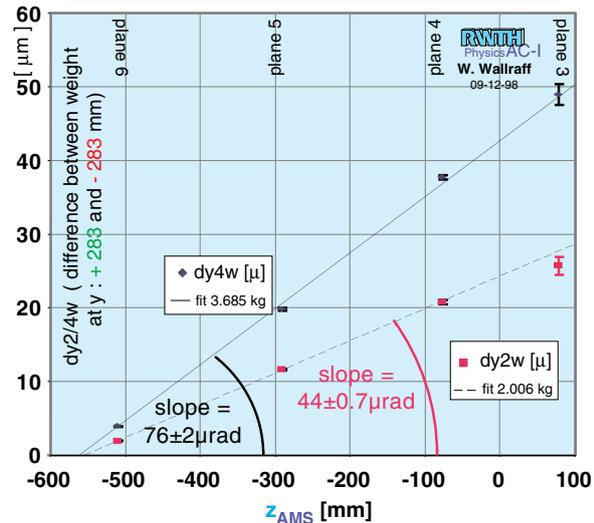
Fig. 3b Measured sloping angle at laser beamports under asymmetric load (details see text)
