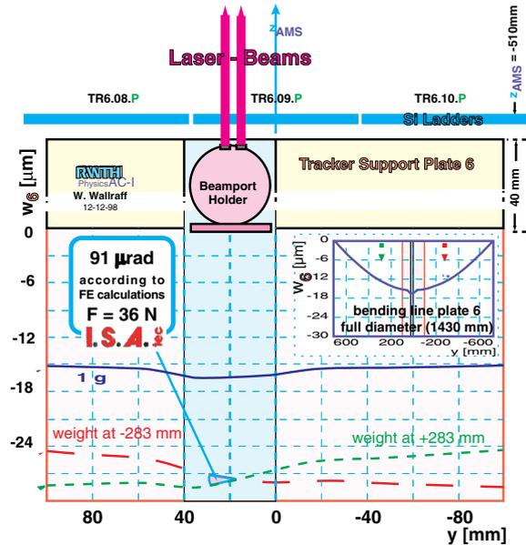
Fig. 3a Laser beam port and Laser/Tracker support plate; bending line unloaded (1g), loaded at +283mm (dotted), loaded at -283mm (dashed), FE model; insert shows full bending line, arrows mark the load positions.
