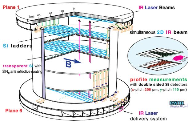
Fig. 1 AMS-01 Si tracker and the Tracker Alignment System. The insert shows laser profiles observed while AMS was in orbit.
