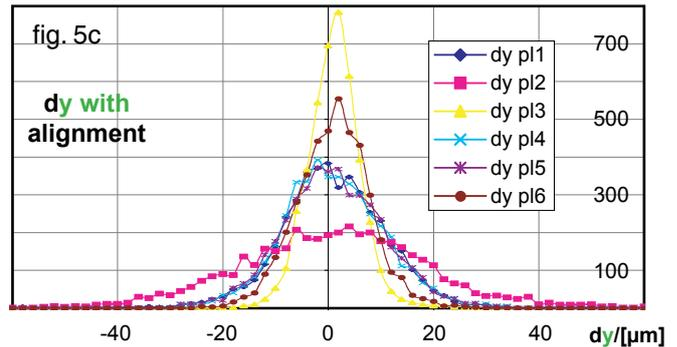
Fig. 5 Frequency distributions of single plane displacement measurements with stiff cosmic tracks (see text). a) [ b, c ] parallel [orthogonal] to **B**.
