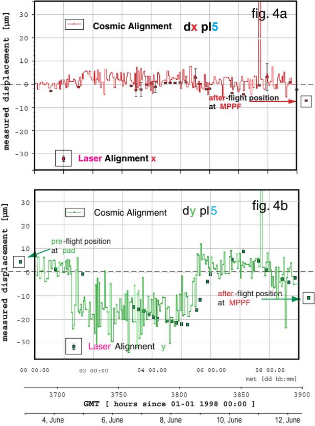
Fig. 4 Measured (see text) time evolution of plane 5 displacements. x (y) parallel (orthogonal) to main B component. The glitch in the early morning of June 11th is excluded from AMS physics data.
