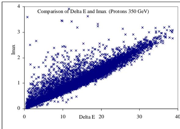
**Figure 6.** Comparison of Imax and  $\Delta E$  for protons at 350 GeV.
