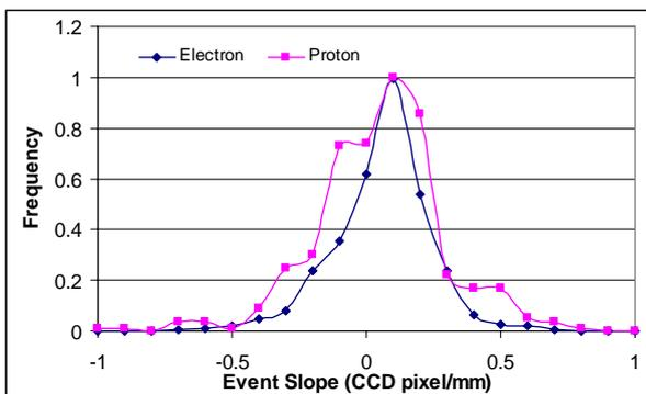
**Figure 7.** Trajectory reconstruction distribution for electrons and protons.
