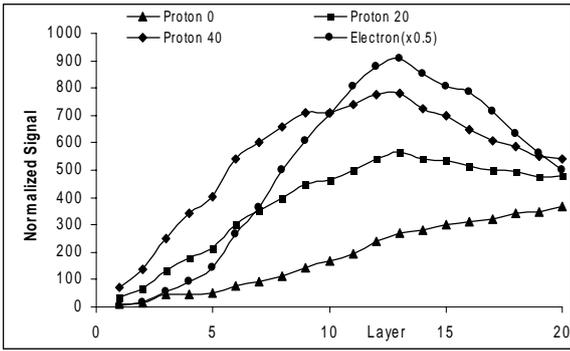
**Figure 2.** Average layer signal in the calorimeter for protons (350GeV) and electrons (150GeV) normally incident. The target thickness for each case is given in the legend in centimeters.
