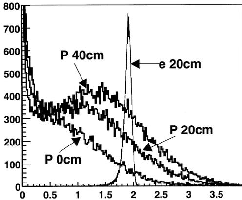
**Figure 3.** Energy Distribution for protons and electron in Figure 2. The energy scale is GeV.
