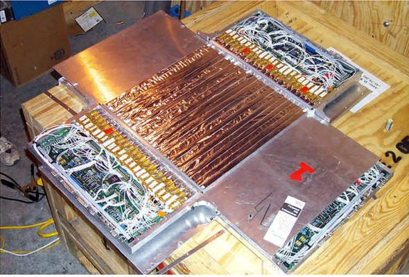
**Fig. 1:** Top view of one half of a hodoscope plane
