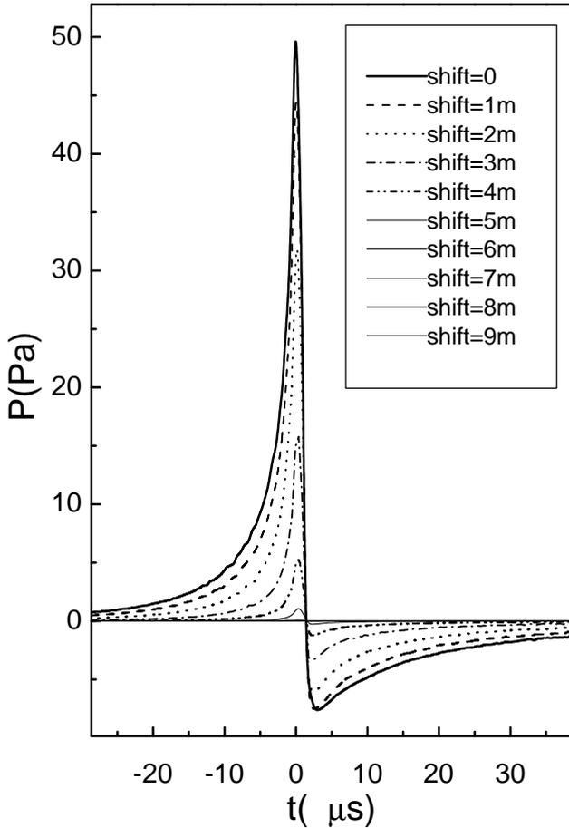
**Fig. 1.** Acoustic pulse amplitudes at an equivalent distance of 1 m from a  $10^{20}$  eV electron-hadron cascade axis. Various offsets from shower maximum are indicated.
