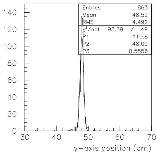
**Fig. 6.** Position resolution,  $\delta x$ , of the extrapolated point of impact in a plane 20 cm above the calorimeter.
