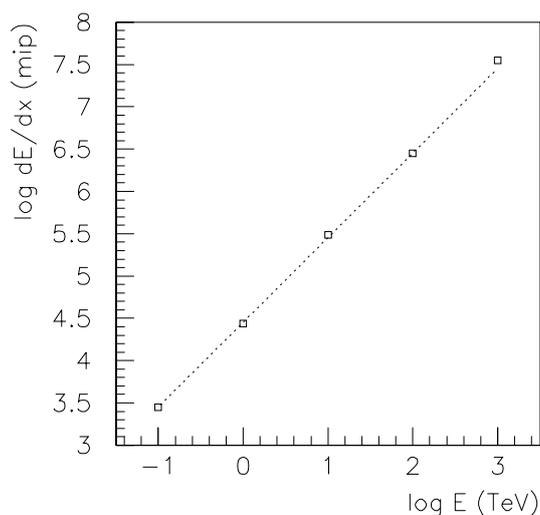
**Fig. 5.**  $dE/dx$  within 5 Si strips vs. initial energy of the proton, 0.1 TeV to 1,000 TeV.
