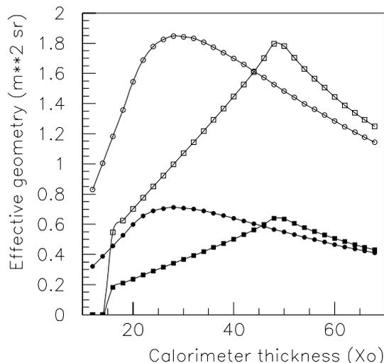
**Fig. 1.** Effective geometric factor vs. calorimeter thickness for protons (circles) and electrons (squares). 2,720 kg (open marks) and 1,156 kg (solid marks) configurations.
