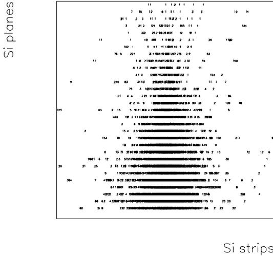
**Fig. 3.** Interaction pattern of a 1,000 TeV proton in the calorimeter.
