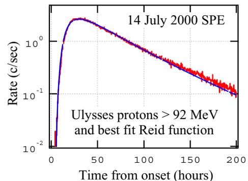
**Fig. 1.** Reid function fit to  $>92$  MeV protons observed by *Ulysses* in the 2000 July 14 SPE. Data are 15-minute averages. *Ulysses* was at 3.2 AU and  $S62^\circ$  at the time.
