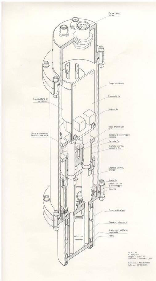
Fig. 1 Schematic of one module of the detector unit
