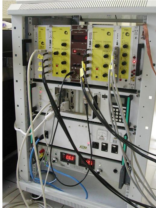
Fig. 2 The electronic and the battery supply units and the computer box
